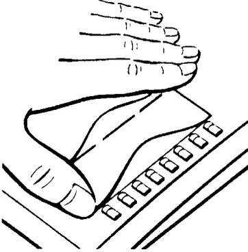
To label the fixed function keys → page 3, punch out the **small** pre-printed labeling card. Insert the card and cover it with the plastic foil supplied (matt side up), as shown in the drawing.
